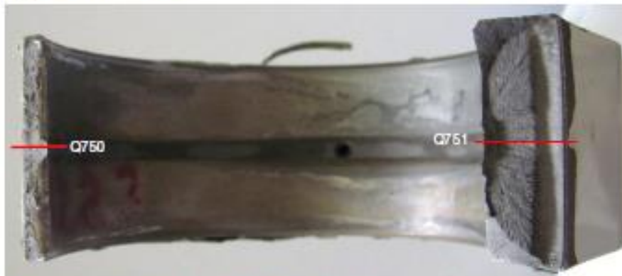
Figure 2: fuse (left) and secondary (right) fracture surface, microsection planes & numbers indicated by red lines
