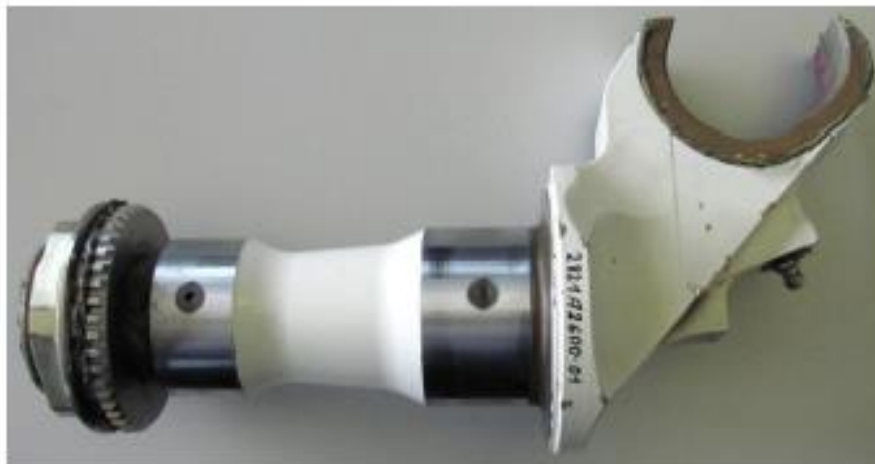
Figure 1: broken Crank Bolt
