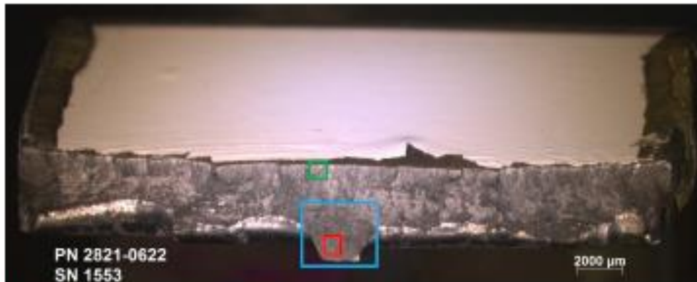
Figure 8: Stereo microscopy photo: fracture surface of the fuse
