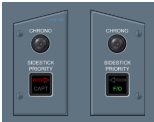
Figure 3: The F/O has the priority and the Captain moves the sidestick
