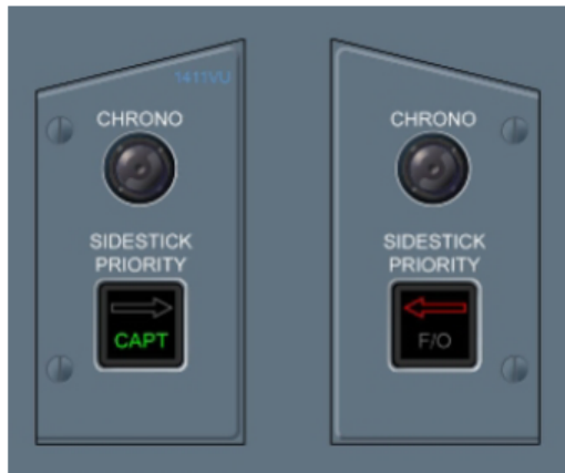
Figure 2: The Captain has the priority and the F/O moves the sidestick
