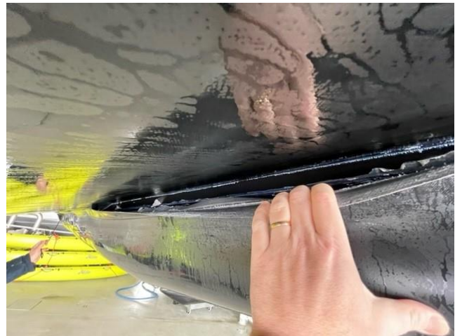
Figure 69: Glue separation at futura tube of Zodiac 12. Photo: Ship management company
