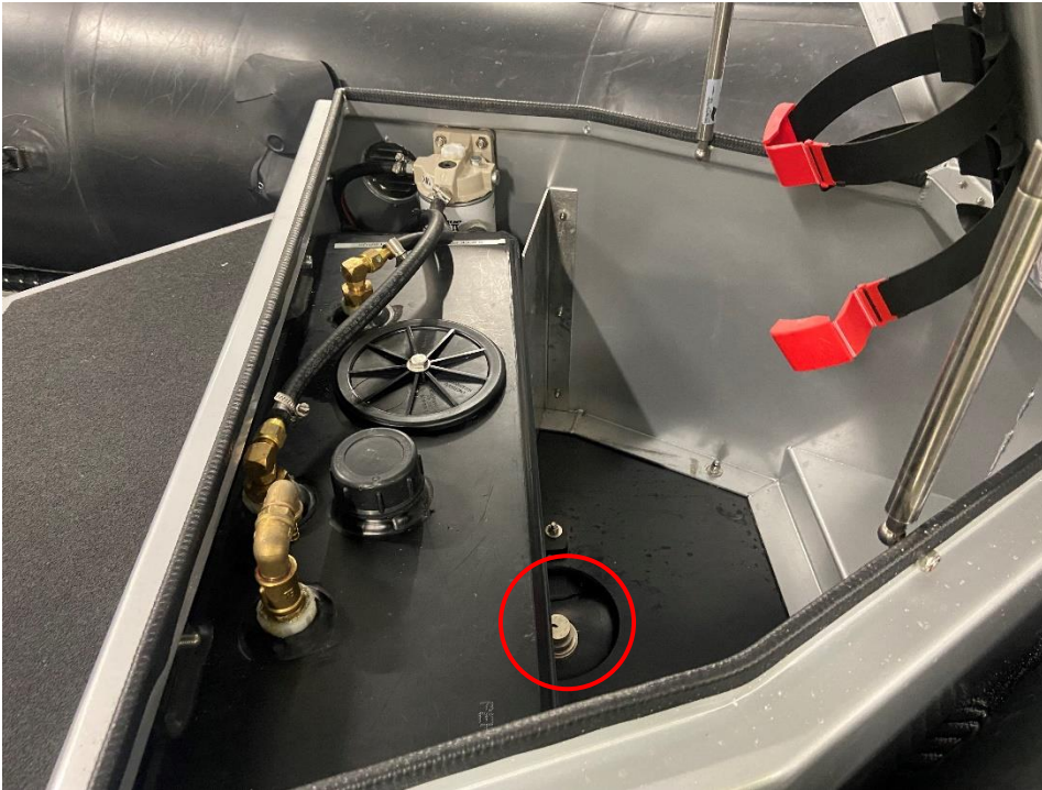
Figure 67: The aluminium box at the bow of one of the Zodiacs. The valve for the inflatable keel is indicated by a red circle. Photo: NSIA
