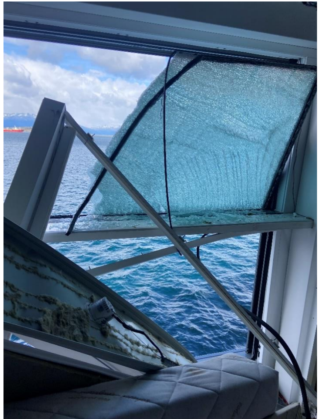
Figure 27: Broken window in stateroom 2016. Photo: NSIA
