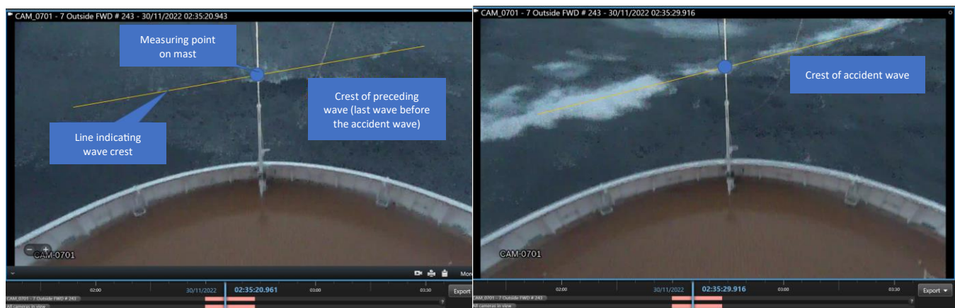
Figure 11-4 CCTV footage from the bridge showing the time interval between the preceding wave and the accident wave, measured from the bow mast.
