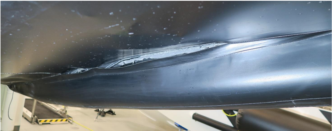
Figure 44: Glue separation damage on the futura tube. Photo: NSIA
