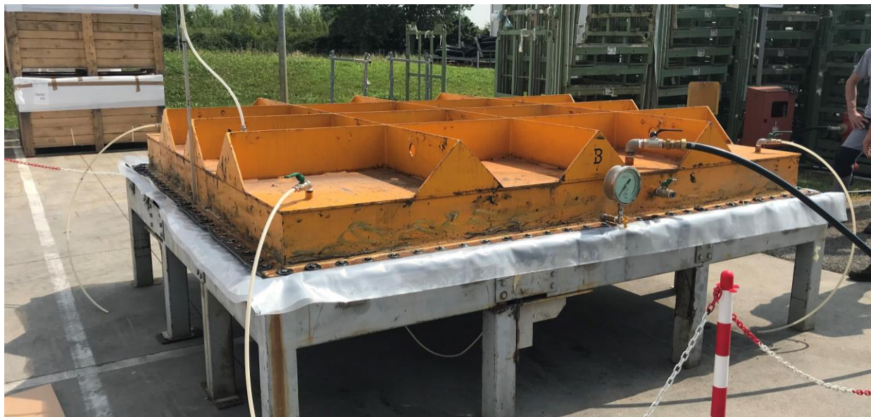
Figure 10-1 Static pressure test. Photo from window manufacturer SOMEK
