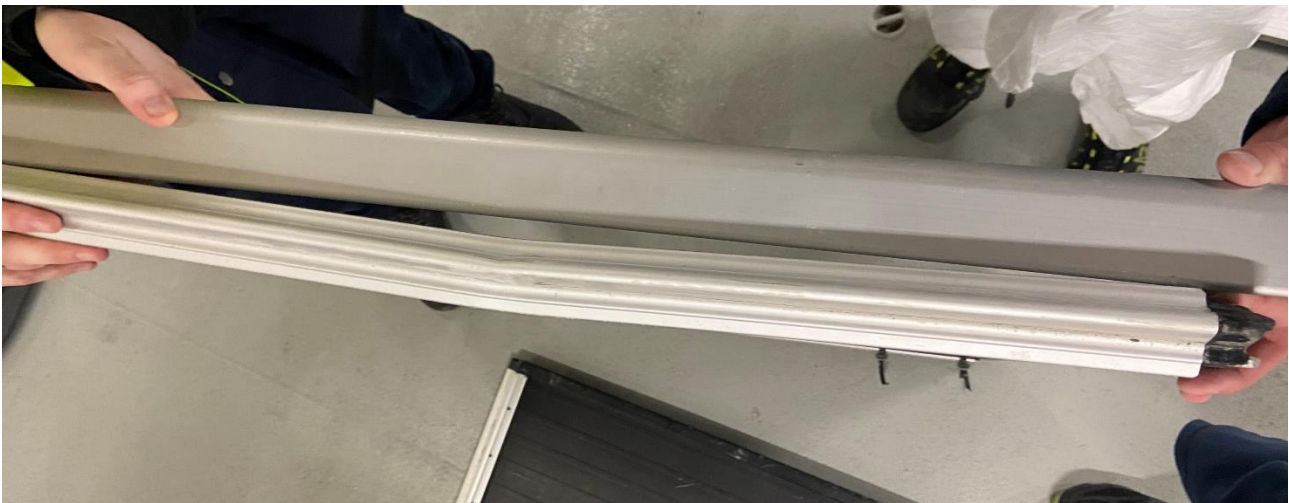
Figure 43: The floorboards in the damaged area were bent. Photo: NSIA
