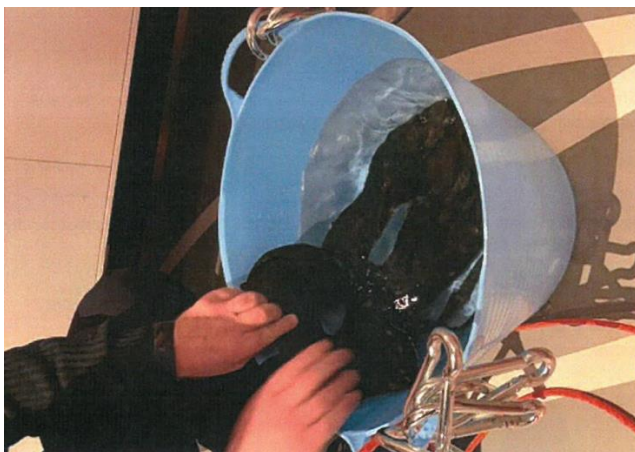
Figure 83: Lifejacket being lowered into a bucket. Photo: Crew
